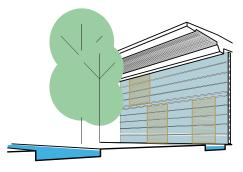
A lake was introduced on the site to aid in sustainable water management, providing rainwater attenuation ensuring that surface water run off doesn't surcharge local sewers.
