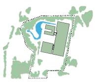
The building was designed with a green roof to reduce visual impact, increase biodiversity and capture rainwater to slow down surface run off. The spoil from construction was used to build the landscape up around the building to screen it from view and to integrate it in to the landscape.
