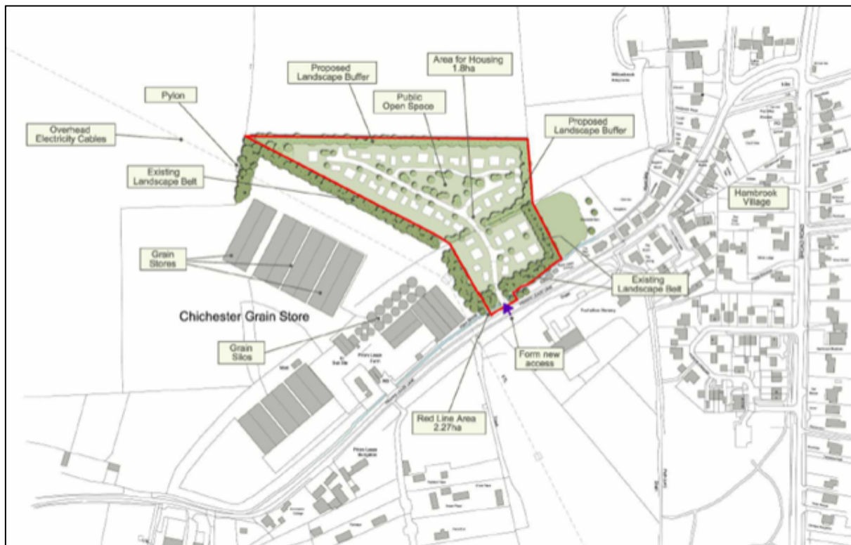
Figure 2. A preliminary layout plan for development at Land at Chichester Grain, Southbourne, reproduced courtesy of Henry Adams LLP.
